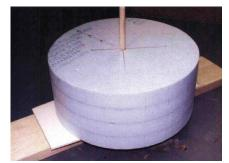
First cut four  $12\times12$  inch squares from the blue foam sheet, and glued them together with the 3M Super 77. The adhesive does not interfere with the sanding of the foam plug. I used my drill press to drill a ½ inch hole in the center of the foam block and then glued the dowel in the center of the block leaving 3/4 –inch sticking out of the bottom and about 3 inches protruding at the top of the block. The dowel will act like a spindle so it must be plumb to the top of the block.
